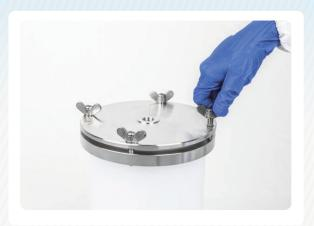
**Step 11** Insert the butterfly bolt to secure the end cover.
