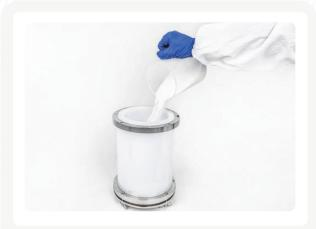
**Step 7** Fill suitable chromatographic media or solid samples into the tube according to user needs.
