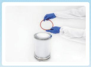
**Step 9** Place the other sealing ring in the groove of the column body opening.
