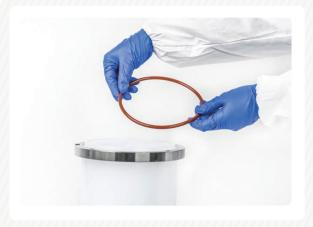
**Step 2** Place the column tube on the lab bench, and place the sealing ring in the groove of the column tube opening.
