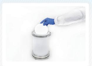
**Step 6** Rotate the column body so that the other opening end is up. Place the bottom frit into the lower part of the column body, and use the plug tool to flatten the bottom frit. At this time, the bottom frit is in contact with the cap.
