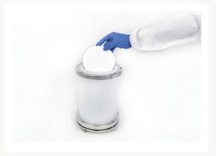
**Step 8** Place the top frit on the filled media bed and align the frit horizontally.
