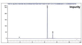
Figure 4. The analytical HPLC chromatogram of the raw sample, the target product and the impurities.
