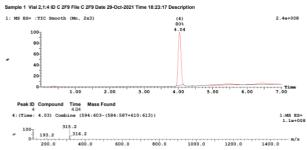
In the LC-MS of the THC fraction, the main THC peak appears at 4.57 mins, with molecular ion M+H $^+$  (m/z. 315.2).
