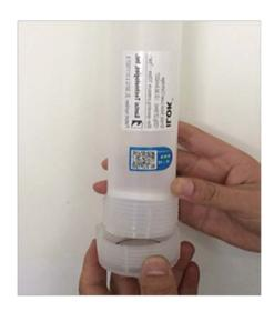
Invert and tighten the i-LOK column.
